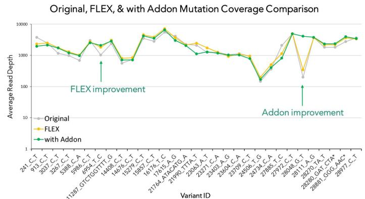
Panels were run in triplicates using a synthetic control (B.1.1.7). Variants were called against the reference genome NC\_045512.2. All 36 mutations were covered and accurately called in each panel tested. Improvements of coverage in FLEX and with Add-on Primers are highlighted above.
